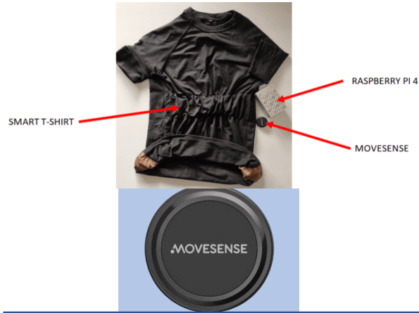
Smart textile with movesense for measurement of ECG and IMU (accelerometer, Gyroscope, Magnetometer)
